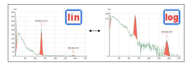
• Toggle channel/keV axis – switching between keV and channel units of X scale
