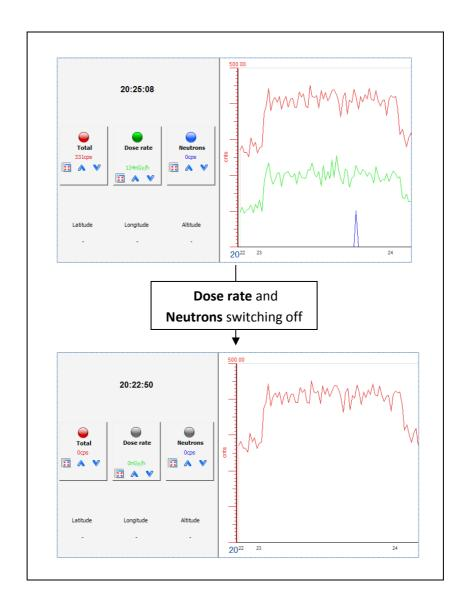
To change Y scale for every profile there are two small buttons (up/down) on each profile button. Clicking on these buttons user adjust Y scales of each profile ( here is the example of this function on Dose rate profile).
