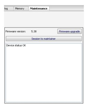
Firmware actualization - to check a current firmware version click on icon Settings on toolbar → in tab Maintenance
