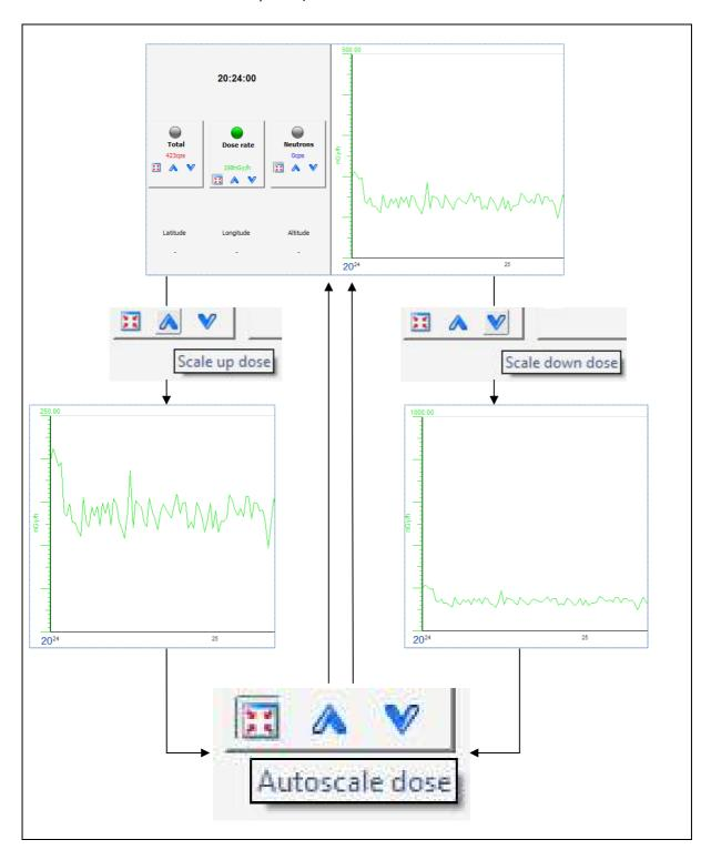
**Reading of Current value** on profiles is joined to mouse cursor. Moving it over profile Total, Dose Rate and Neutrons are proportionally updated in respect to x position of the cursor.
