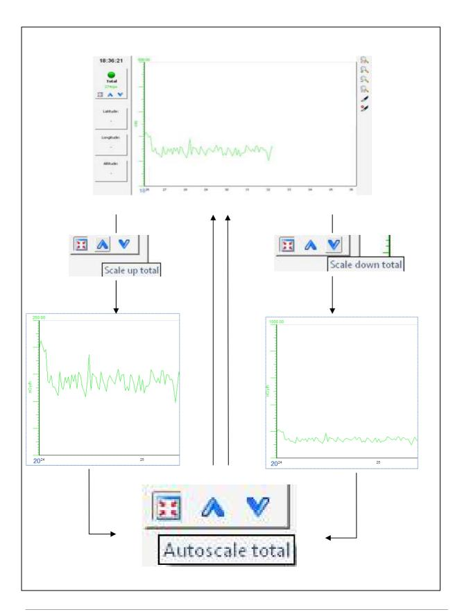
• **Reading of Current value** on profiles is joined to mouse cursor. Moving it over profile Total, Dose Rate and Neutrons are proportionally updated in respect to x position of the cursor.
